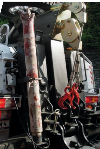
mount for cardan shaft on the support foot
