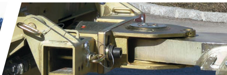
bar eye adapter in different sizes (NATO connection)
